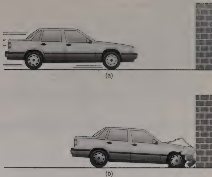
Figure 1.6 Strain in the real world. (a) A sedan approaches a brick wall in a crash test, and (b) the same sedan after impact. Note the extreme distortion of the front (i.e., inhomogeneous strain distribution).
