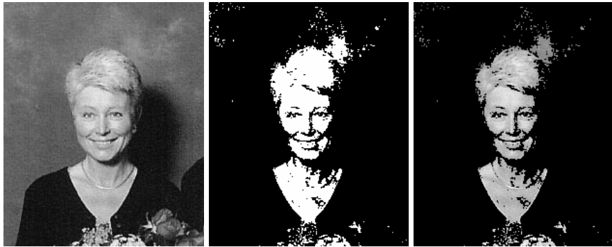
Figure 8.13 Source Image, the Mask Resulting from Compare , and the Result of CopyWithMask
