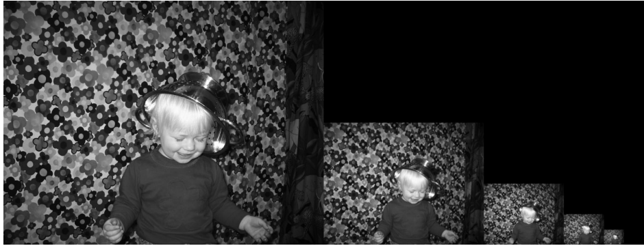
Figure 12.9 A Composite Image of a Five-Level Gaussian Image Pyramid
