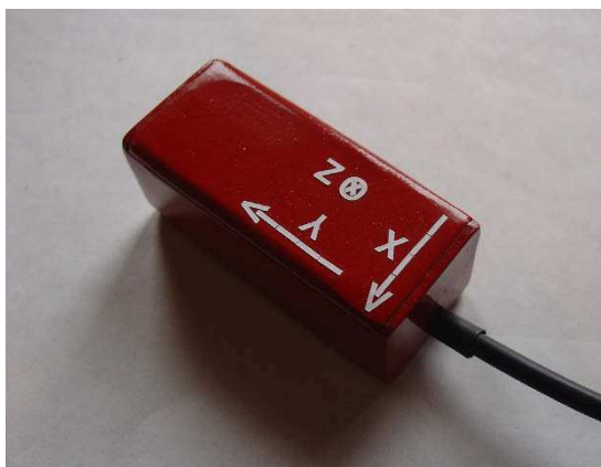
Fig.41 The accelerometer MMA7260QT, accommodated on the sensor board
