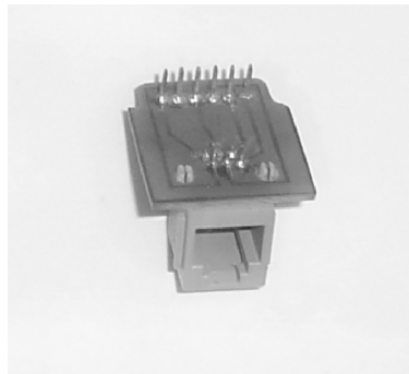
Figure 3.23 Breadboard adapter for 6P6C connector
