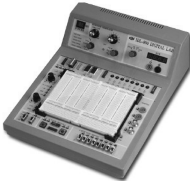
Figure 3.22 IDL-800 Digital Lab breadboard.
