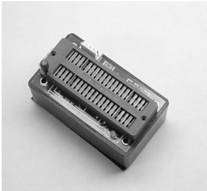
Figure 1.1 USB PIC programmer made by MicroPro.
