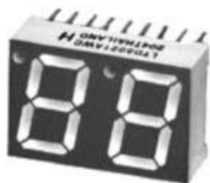
Figure 5.14 A 2-digit 7-segment display
