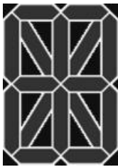
Figure 1.6 16-segment LCD display
