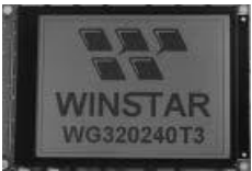
Figure 1.8 Graphics LCD display
