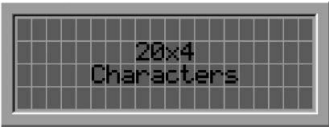
Figure 1.7 Dot matrix LCD display
