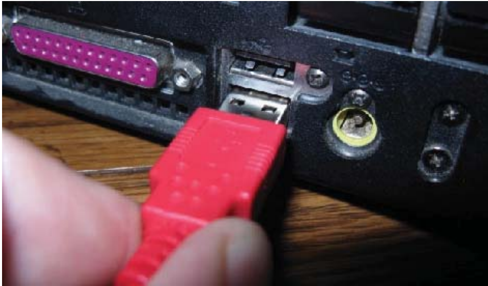
FIGURE D.4 Pictorial view of connecting the PICkit™ 3 to the USB port.
