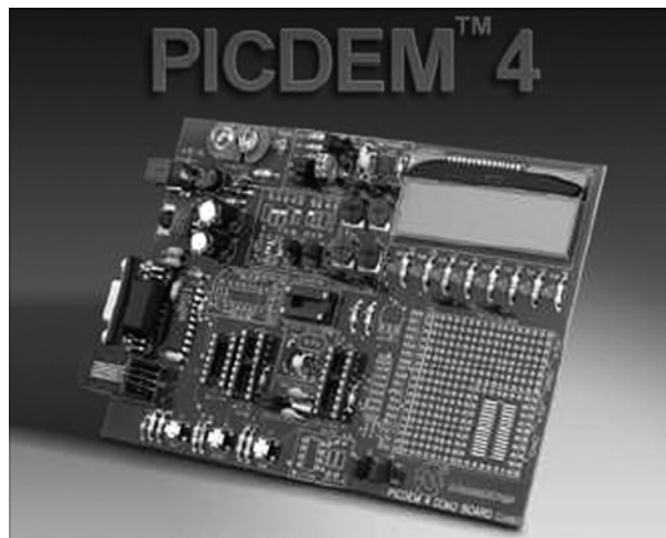
Figure 5.3: PICDEM 4 development board
