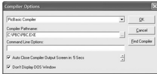
Figure 3.21 Configuring CodeDesigner Lite for the PicBasic compiler
