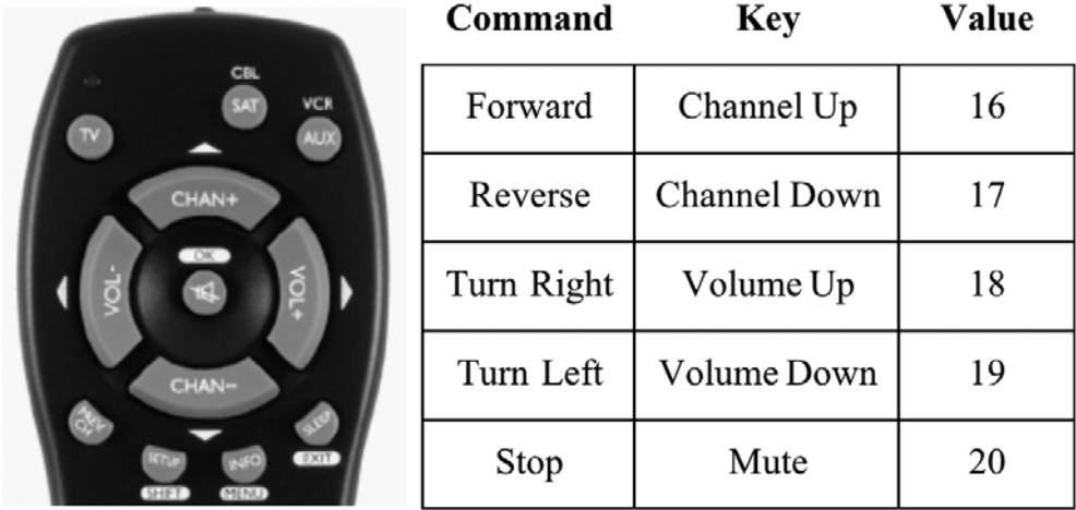
Figure 18-6 TV remote control and commands used in Experiment 3
