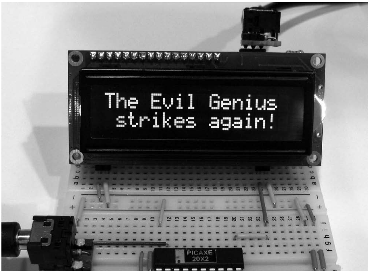
Figure 10-5 Breadboard setup for completed serial LCD project
