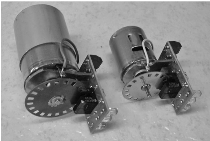
Figure 15.1 Small DC electric motors with encoders that show simple two phase, quadrature encoders and encoder readers attached to them.
