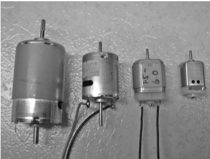
Figure 14.1 Examples of small DC motors under discussion. Motors with shafts on both ends will allow us to mount an encoder directly on one end for later experiments.
