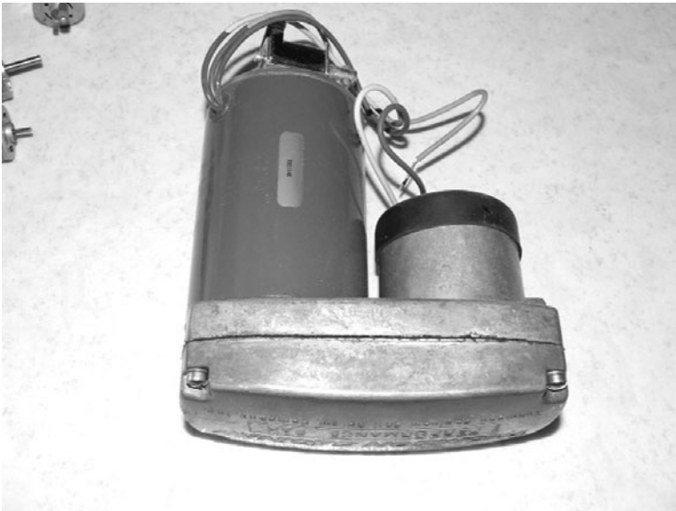
Figure 17.1 A small fractional HP AC motor with an integral drive unit
