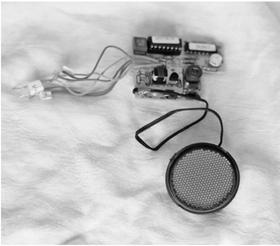
Figure 21.8 The Polaroid 6500 ultrasonic ranging module.
