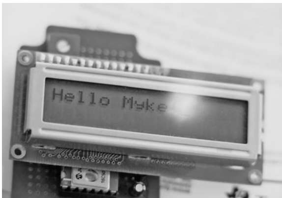
Figure 21.6 The serial LCD interface in operation.
