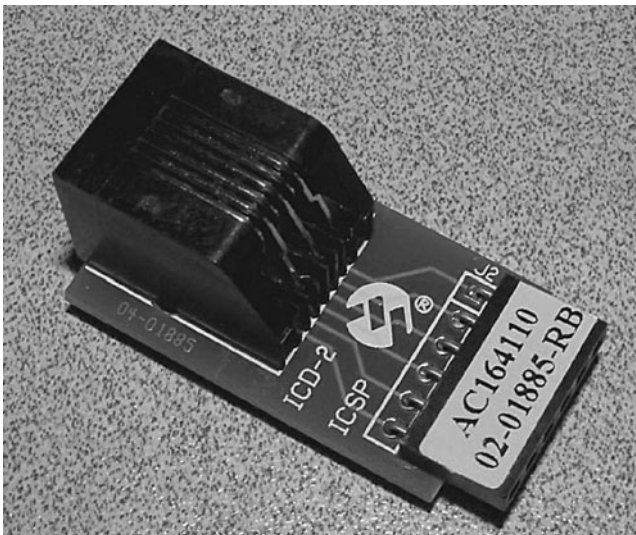
Figure 5.11 The Microchip ICD 2 to ICSP adapter (part number AC164110) is an easy way to use the MPLAB ICD 2 debugger with breadboarded applications.
