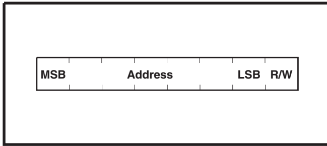
Figure 9-2 Phillips I2C 7-bit address specification
