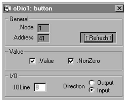
Figure 4-5 The button object when no button is pressed
