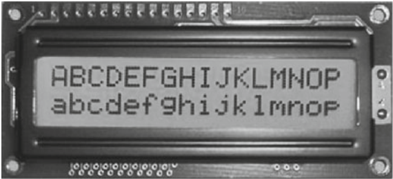
Fig. 8.46 A common 2 × 16 alphanumeric LCD module
