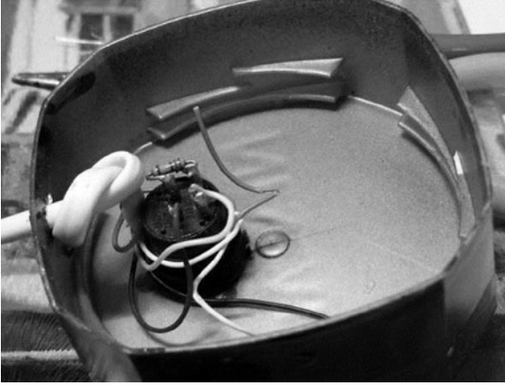
Figure 3-7. The coffee jar lid button mount
