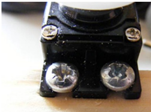
Figure 4-6. Using self-tapping cheesehead screws
