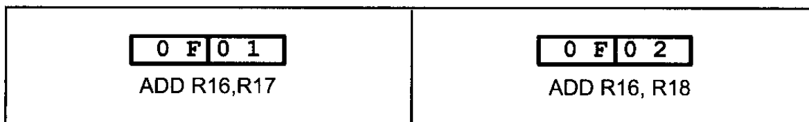
Figure 2-17. The Machine Code for Instruction “ADD Rd,Rr” in Hex
