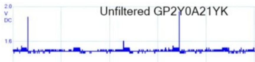
Figure 2.31. Noise on a GP2Y0A21YK IR distance sensor shows large periodic spikes.
