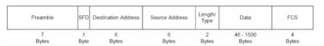
Figure 9.22. An Ethernet frame can hold 46 to 1500 bytes.
