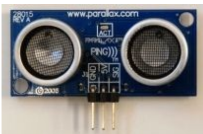
Figure 10.10. An ultrasonic pulse-echo transducer measures the distance to an object, Ping))).
