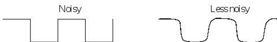
Figure 10.24. Limiting rise/fall times can reduce radiated noise.
