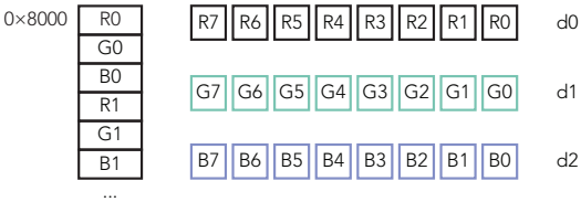
FIGURE 8-2: Loading RGB data with a structured load
