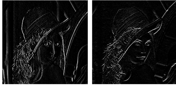
■ FIGURE 4.4 I_x (left), I_y (right) of Lena image using Sobel filter.
