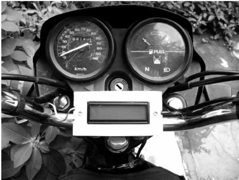
Fig. 6: Speedometer-cum-odometer unit on a bike's handle bar
