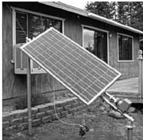
Fig. 5. Solar module (without LDR) mounted on the support system (courtesy: www.livingonsolar.com )
