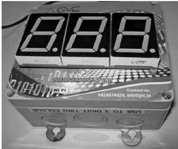
Fig. 7: Author's prototype of traffic light count-down timer with dual-colour display
