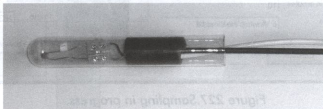
Figure 228. Outdoor sensor in a protective tube.
