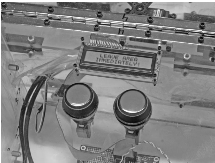
Figure 11-23 The room board LCD display when unsafe air conditions are detected.
