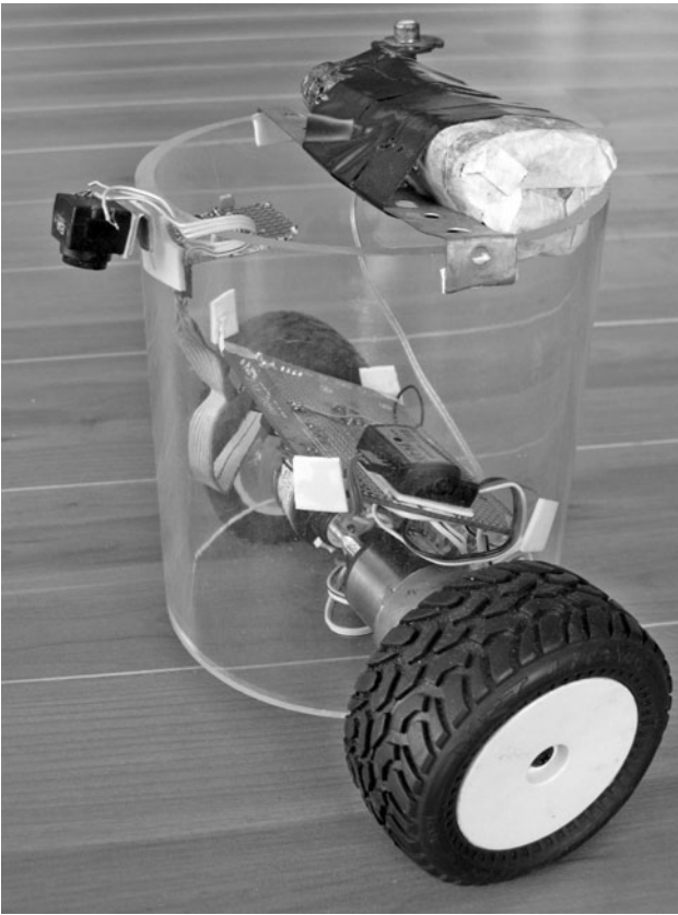
Figure 7-9 DanceBot with camera configured to follow lines.
