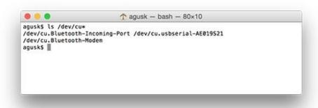
My Foca serial adapter was recognized as /dev/cu.usbserial-AE019521 on my OSX.
